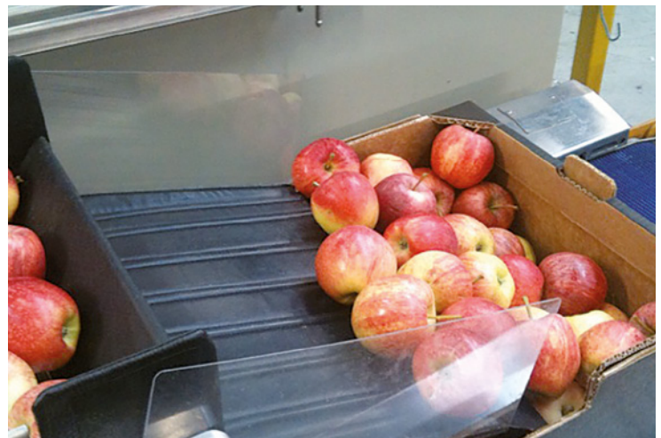
Soft filling support of loose fruits in boxes
